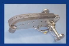
CfC monoblock and W brush armoured vertical target (EU).
